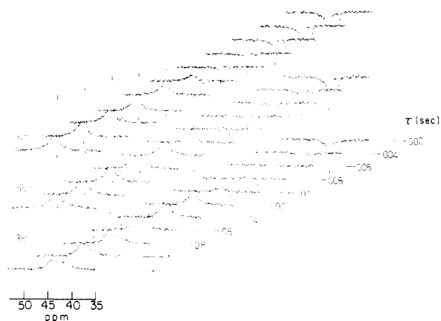
FIGURE 6: Inversion-recovery measurement using a D = 180^\circ - \tau - 90^\circ pulse sequence of the T_1 values of the three cell wall ^{13}\text{C} resonances of ^{13}\text{C}_2 -Gly-labeled S. aureus cell walls at 35, 55, and 75 °C. Signal amplitudes were obtained from computer-simulated band shapes (not shown). A delay, D , of 4 s ( > 5T_1 ) was used in each measurement.
